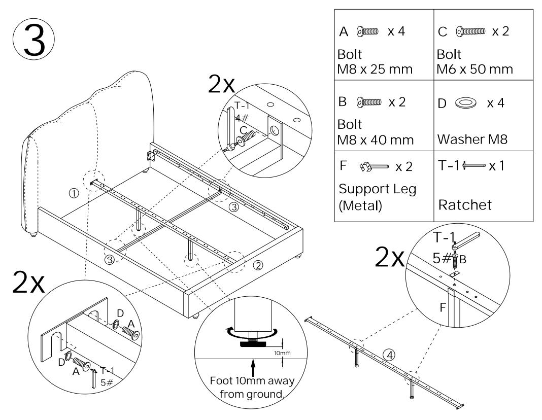
ATTENTION: After central rail and support legs have been assembled, rotate adjustable feet to make support legs 10mm away from the floor. Support legs would touch the floor when a mattress is put on the base.
