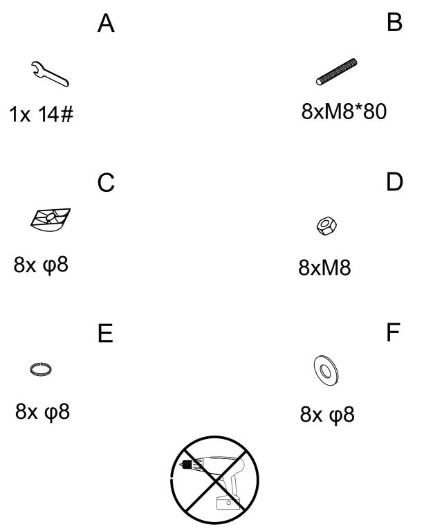
We strongly advise that you do not use Power Tools, such as drills or electric screwdrivers during the assembly as this may cause irreparable damage and will invalidate your warranty.
